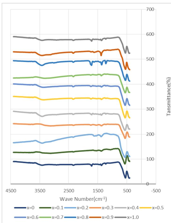
Fig (4). The IR absorption spectra of  $Mg_{1-x}Zn_xFe_2O_4$  ferrites.
