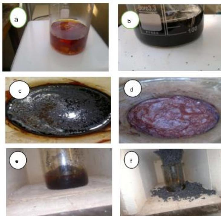
Figure (1): Photograph of (a) nitrate-citrate solution, (b) The solution after the Adding of ammonia, (c) dry gel, (d) Dry bulk temperature of 120<sup>0</sup>C, (e) ) Dry bulk temperature of 220<sup>0</sup>C and (f) auto combustion and become Nano powder ferrite
