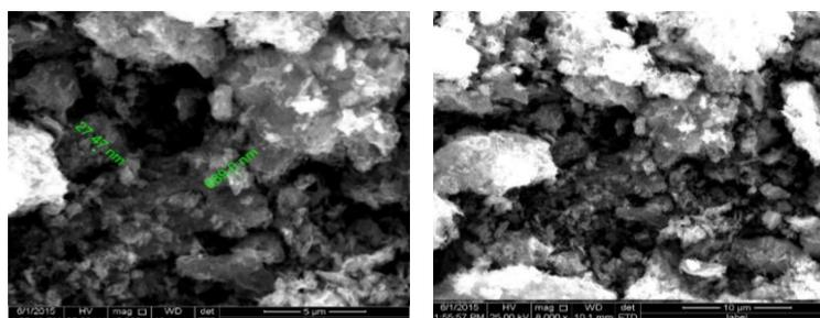
Figure(2). SEM micrographs for  $Mg_{0.5}Zn_{0.5}Fe_2O_4$  prepared at 220<sup>0</sup>C.
