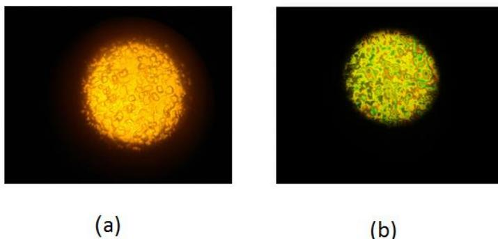
Fig. 4: The wafer of p-type silicon with amplification by 600 times for the internal composition of the (a) before the thermal oxidation (b) after cleaning and thermal oxidation with maximum temperature ( $1200^{\circ}\text{C}$ ).
