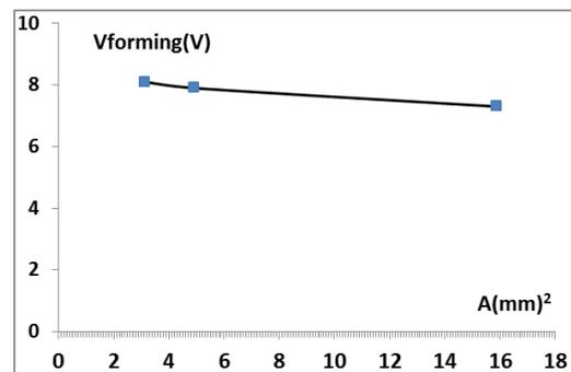
Fig. 9: The relation between A and  $V_{\text{forming}}$  for many devices with CuO coating.
