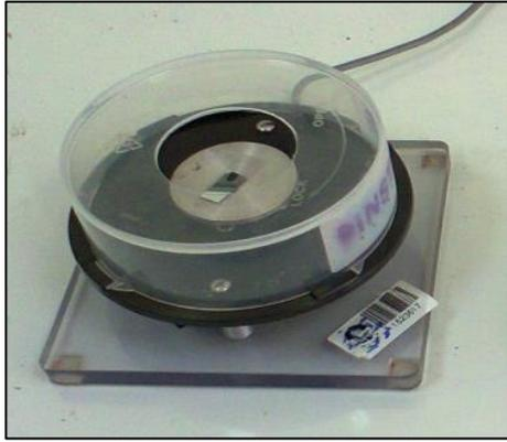
Fig. 5: The images of The Spin-Coater for thin films polymers.
