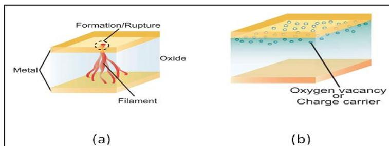
Fig. 3: Schematics (a) resistive switching of a filament conducting track, (b) resistive switching of an interface. conducting track. [9].
