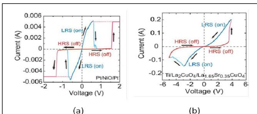
Fig.2: I - V curves during different type of resistive switching: (a) unipolar switching in a Pt/NiO/Pt cell and (b) bipolar switching in a Ti/La<sub>2</sub>CuO<sub>4</sub>/La<sub>1.65</sub>Sr<sub>0.35</sub>CuO<sub>4</sub> cell. [9].
