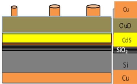
Fig. 7: The cross section of the structures.
