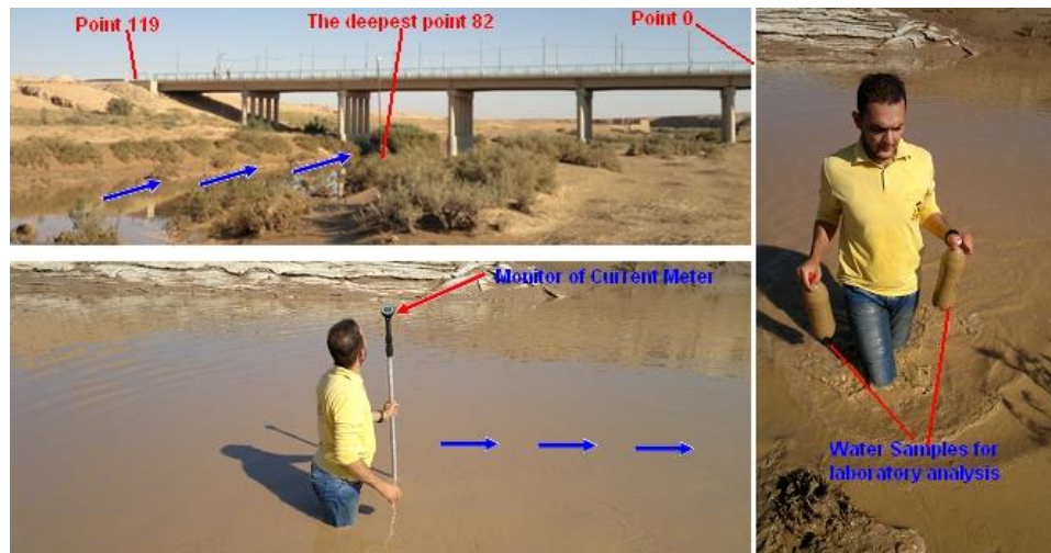
Plate (1). describes how to measure the flow velocity by flow meter (bottom left), and sampling of the valley water (right) and survey the observation station on Tharthar valley / Hatra bridge (top-left).
