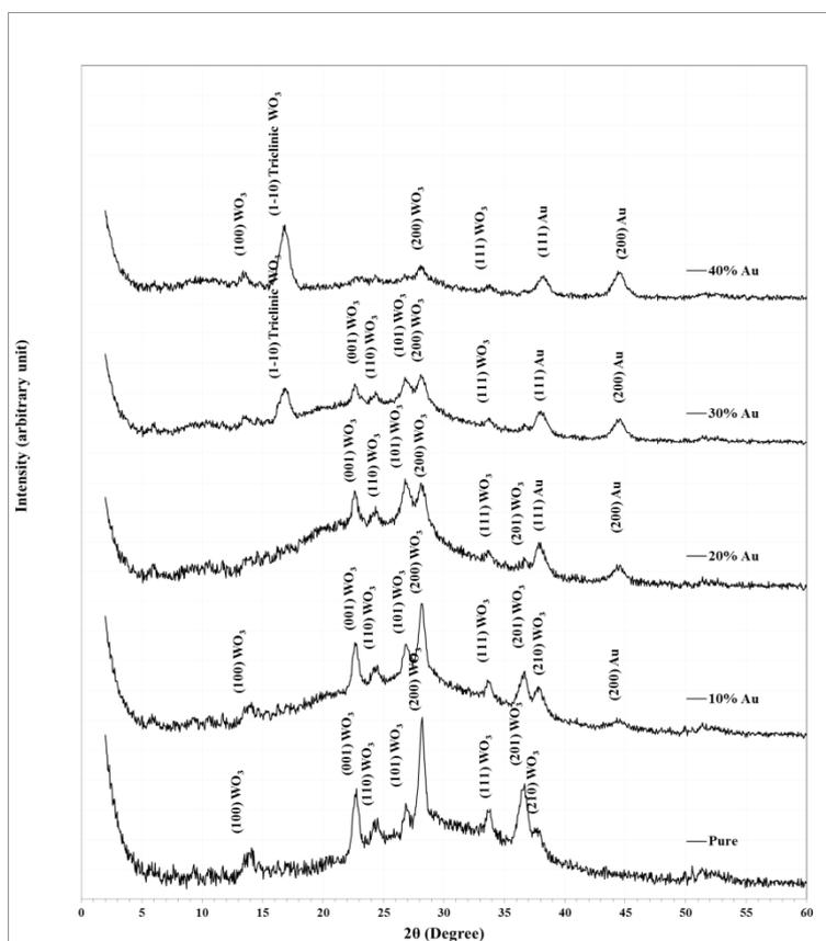
Fig.2: The XRD pattern of  $WO_3$  and doped of Au (0, 10,20,30 and 40) wt. %thin films with annealing temperature at  $T_a = 400\text{ }^\circ\text{C}$ .
