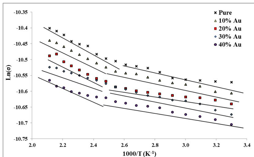
**Fig.3:**The graph shows the variation of  $(Ln\sigma)$  with  $(1000/T)$  for pure  $WO_3$  and doped Au at different concentration on glass substrate as deposited
