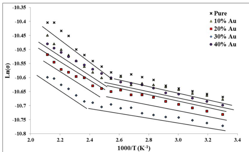
Fig.4: The graph shows the variation of  $(Ln\sigma)$  with  $(1000/T)$  for pure  $WO_3$  and doped Au thin films at different concentration on glass substrate at temperature  $400^\circ C$ .
