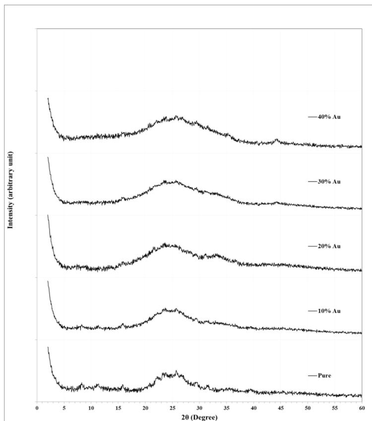
Fig.1 : The XRD pattern of  $WO_3$  doped of Au(0,10,20,30 and 40) wt. % thin films as deposited .
