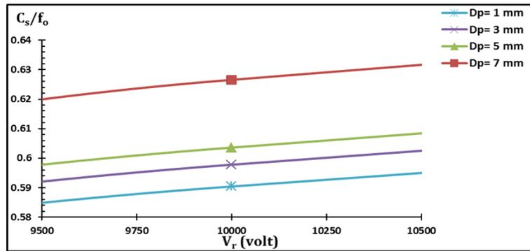
Figure (7): Comparison between the relative values ( $C_s/f_o$ ) of different polepiece bore diameter ( $D_p$ ) with respect to the  $V_r$  at constant excitation of ( $NI = 10$  kA.t).
