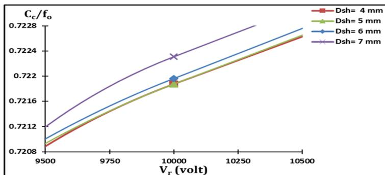
Figure (4): Comparison between the relative values ( $C_c/f_o$ ) of different iron shroud bore diameter ( $D_{sh}$ ) with respect to the  $V_r$  at constant excitation of ( $NI = 10 \text{ kA.t}$ ).
