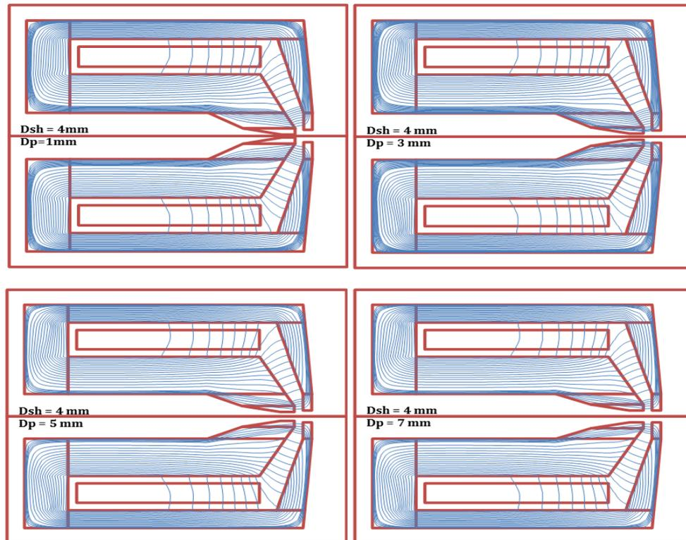
**Figure (10): The geometrical shape models of the objective lenses of ( $D_{sh} = 4 \text{ mm}$ ) and different values of  $D_p$  and their magnetic flux density distributions at constant excitation of ( $NI = 10 \text{ kA.t}$ ).**
