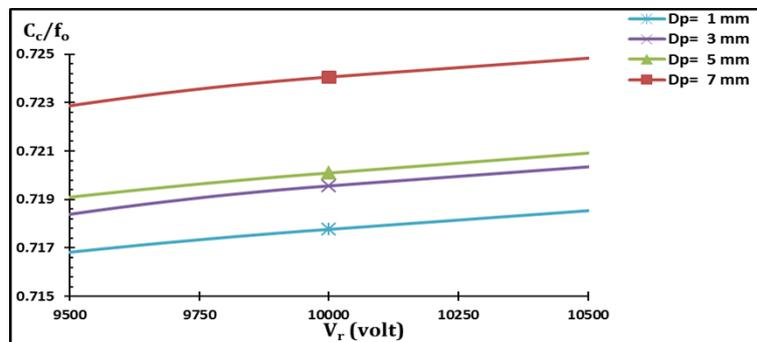
Figure (8): Comparison between the relative values ( $C_c/f_o$ ) of different polepiece bore diameter ( $D_p$ ) with respect to the  $V_r$  at constant excitation of ( $NI = 10$  kA.t).
