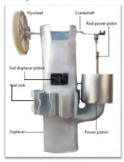
Fig. 3 shows the fabricated of stirling engine
