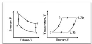
**Fig .1:** *P-V* and *T-S* diagrams for the stirling engine[11]. (1-2) on the P-V and T-S diagrams show the starting point of the cycle. The Piston within expansion space its inner most dead point and the compressed space is
