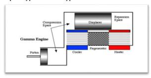
Fig .2 show Gamma Stirling engine type [14].
