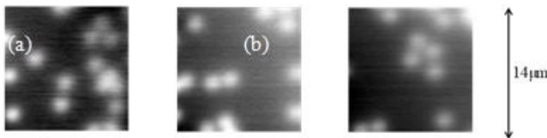
Fig .3. Scanning Hall Probe images of Sr 2 RuO 4 at three different locations. The sample was cooled in the earths filed. [T=300mk, H APP =0]
