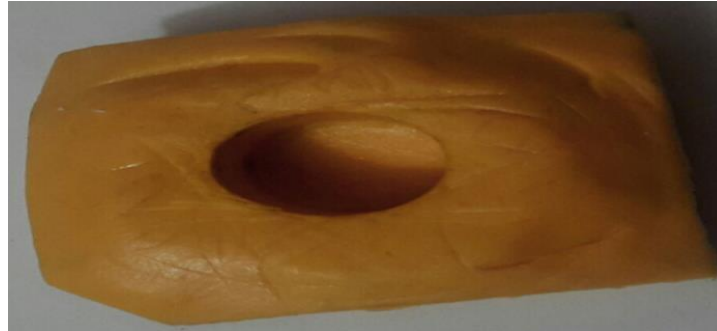
Figure (1) Template used for sample preparation (6 x 10mm)
