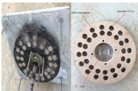
Fig. 3: Shows the magnet Inhibition disc and how to install the rotors magnet for the generator.
