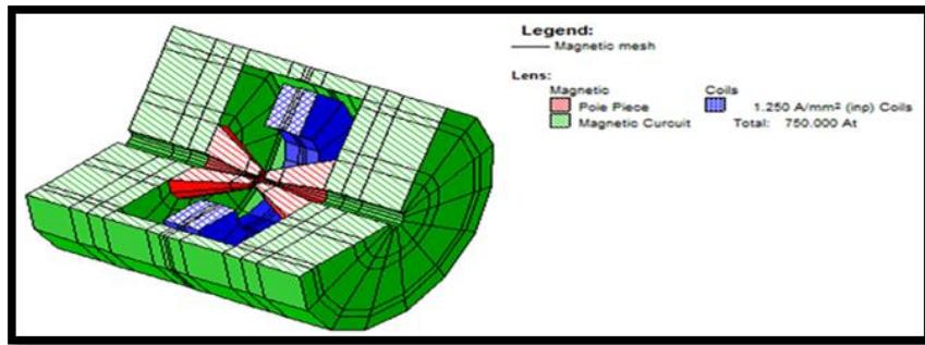
Fig. 2: 3-D magnetic bipolar prototype lens.
