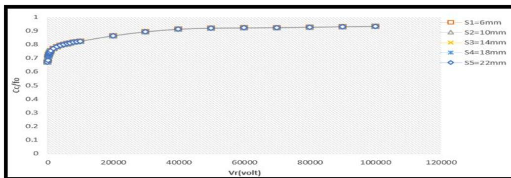
**Fig. 4: Chromatic aberration relative to focal length as a function of relative corrected acceleration voltage  $V_r$  at a current density of ( $\sigma = 6 \text{ A/mm}^2$ ).**
