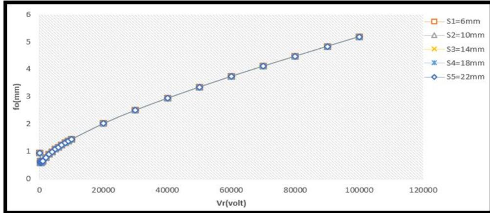
**Fig. 6: Focal length as a function of relative corrected acceleration voltage  $V_r$  at a current density of ( $\sigma = 6 \text{ A/mm}^2$ ).**
