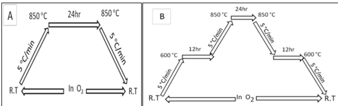
figure (1) A- sintering process, B- annealing process
