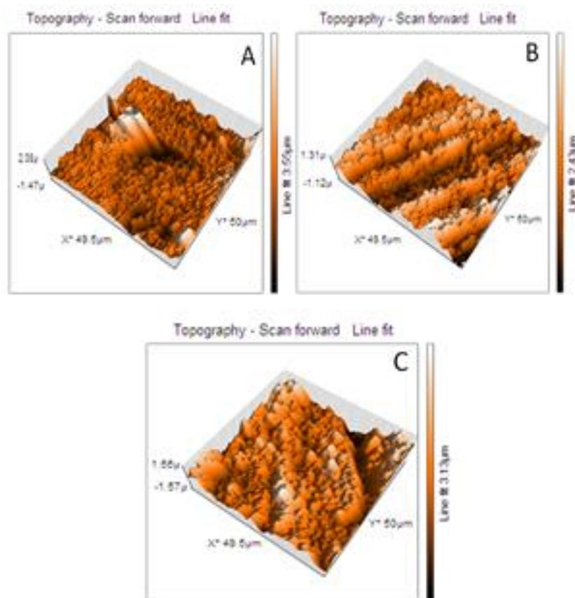
**Fig (7) : AFM surface images of  $(\text{Hg}_{1-x}\text{Pb}_x\text{Ba}_2\text{Ca}_{3-y}\text{Mg}_y\text{CuO}_{10+\delta})$  compound when A- ( $x = 0, y = 0$ ), B- ( $x = 0.4, y = 0$ ), C- ( $x = 0.4, y = 1.4$ ).**
