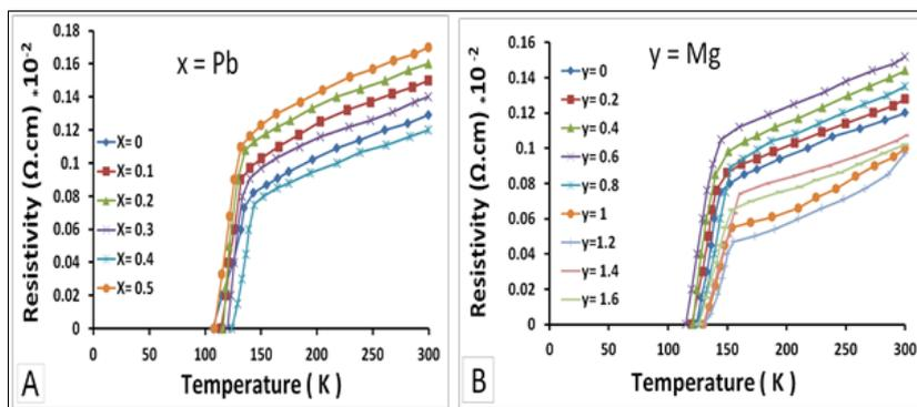
fig (4) Temperature dependence resistivity for  $(\text{Hg}_{1-x}\text{Pb}_x\text{Ba}_2\text{Ca}_{3-y}\text{Mg}_y\text{CuO}_{10+\delta})$  samples when A: (  $x=0,0.1,0.2,0.3,0.4,0.5$  ;  $y=0$ ), B: (  $y=0,0.2,0.4,0.6,0.8,1,1.2,1.4,1.6$  ;  $x=0.4$  ).
