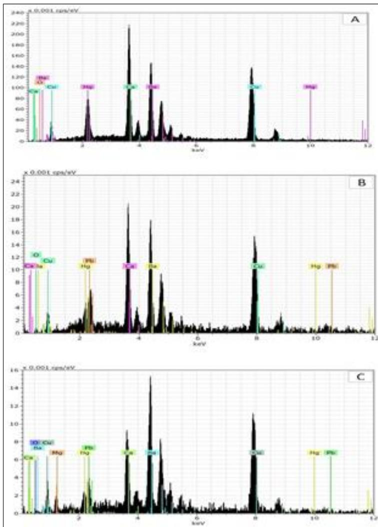
**Figure (5) The EDX pattern for  $(Hg_{1-x}Pb_xBa_2Ca_{3-y}Mg_yCuO_{10+\delta})$  compound when A-  $(x = 0, y = 0)$ , B-  $(x = 0.4, y = 0)$ , C-  $(x = 0.4, y = 1.4)$**
