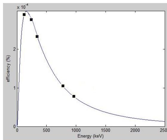
**Fig (3) Eu-152 efficiency curve for the case  $\pm\sigma$**
