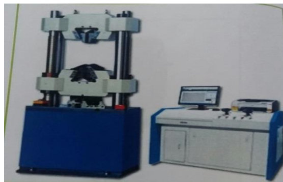
Fig. 1: showing the bending test device
