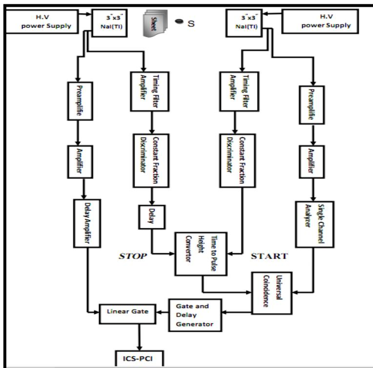
Fig. 1: Block diagram of the gamma-gamma coincidence spectrometer
