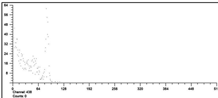
Fig. 5: coincidence Spectrum at the 1332KeV gate.
