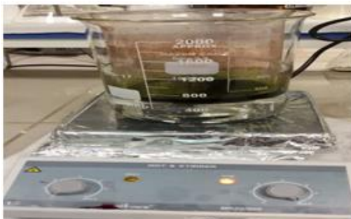
Fig. 2 and 3: Warm steps of oxidation of Graphite
