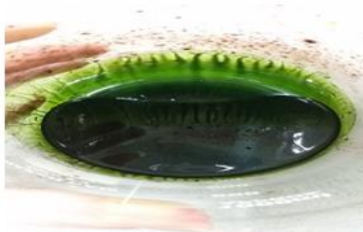
Fig. 2 and 3: Warm steps of oxidation of Graphite
