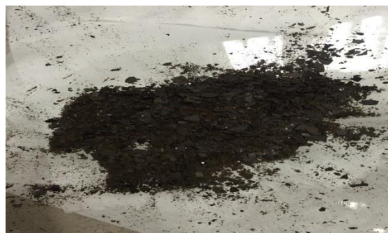
Fig. 5: Filtration steps to find the powder of Graphene Oxide
