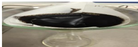
Fig. 7: Filtration of Silanization step of Graphene oxide
