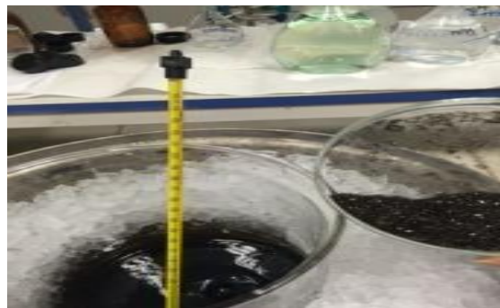
Fig. 1: Cold steps oxidation of Graphite to Graphene and Graphene Oxide
