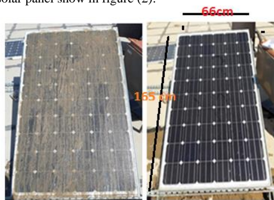
Fig. 2: left Solar panel with dust, right Solar panel clean.
