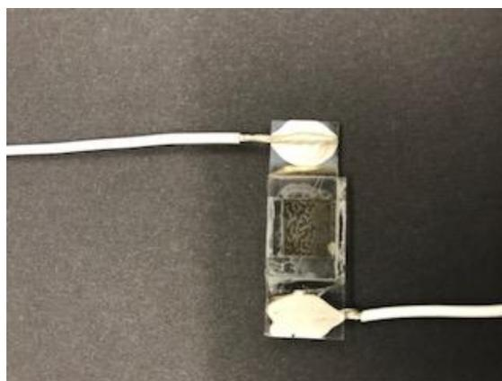
**Fig. 6:** The cell of PDLC (5CB doped with chitosan) doped with SBB dye.
