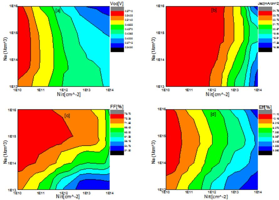
**Fig. 9:** shows the effect of the concentration of  $N_A$  impurities with the density of the interface states on the performance of the solar cell
