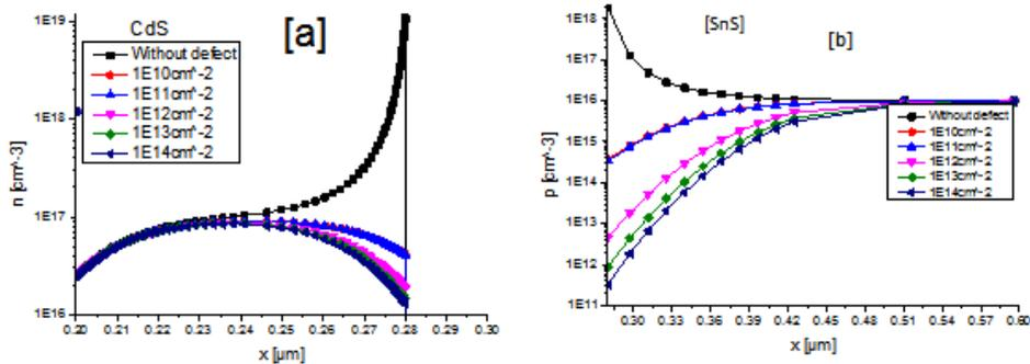
Fig. 4: shows the change in the concentration of charge carriers [a] electrons and [b] holes with the change in the density of the interface states
