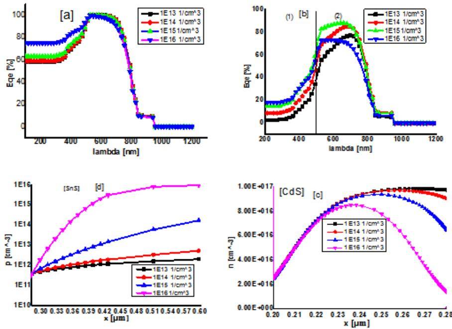
Fig. 10: illustrates [a] the process of recombining carriers within the region of depletion [b] the quantum efficiency at an interface defect density of  $1E14\text{cm}^{-2}$ , [c] and [d] the concentration of the electrons and the holes with the concentration of the  $N_A$  carriers changes
