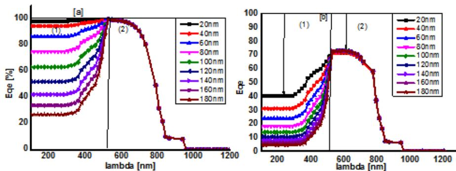
Figure (8) shows the change of quantum efficiency at the density of the interface states [a]  $1E10cm^{-2}$  and [b]  $1E14cm^{-2}$  with the change in the thickness of CdS.
