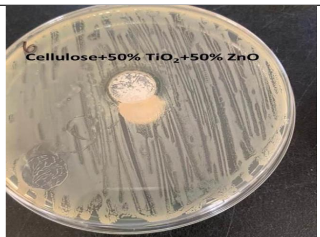
Fig.14 Antibacterial activity of cellulose composite under testing [methylcellulose+50% TiO_2 +50% ZnO].
