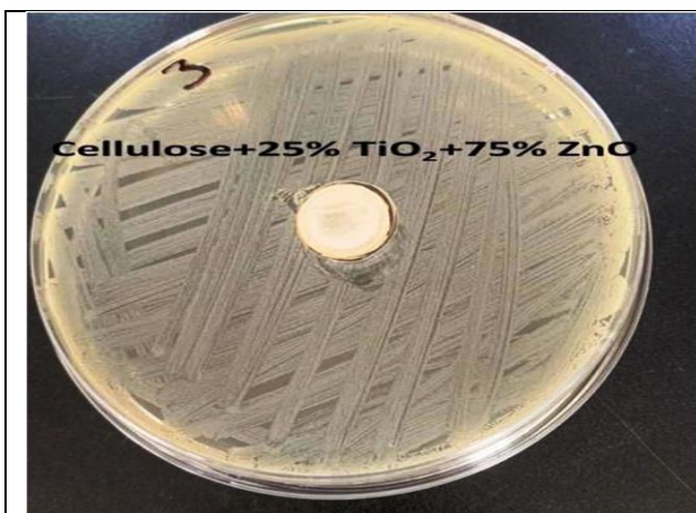
Fig.14 Antibacterial activity of cellulose composite under testing [methylcellulose+25% TiO_2 +75% ZnO].
