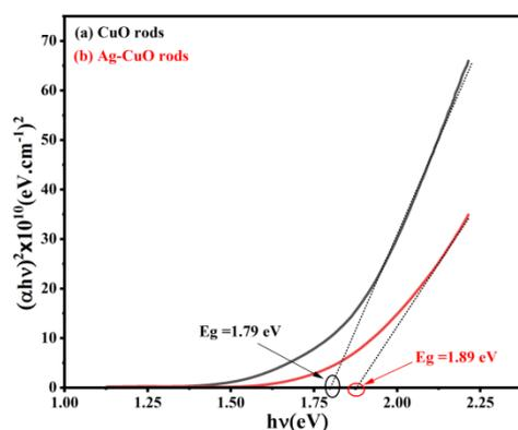
Fig. 4: Tauc's plot: (a) CuO nano-rods deposited on CuO thin layer, (b) CuO nanorods with Ag nanoparticles
