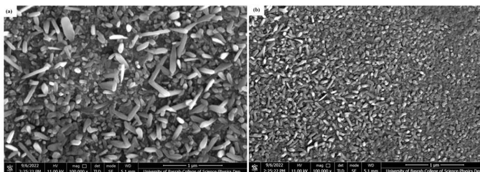
Fig. 2: FESEM images: (a) CuO nanorods deposited on CuO thin layer, (b) CuO nanorods with Ag nanoparticles
