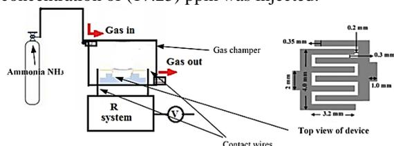
Fig. 1: Schematic illustration of measurement set-up
