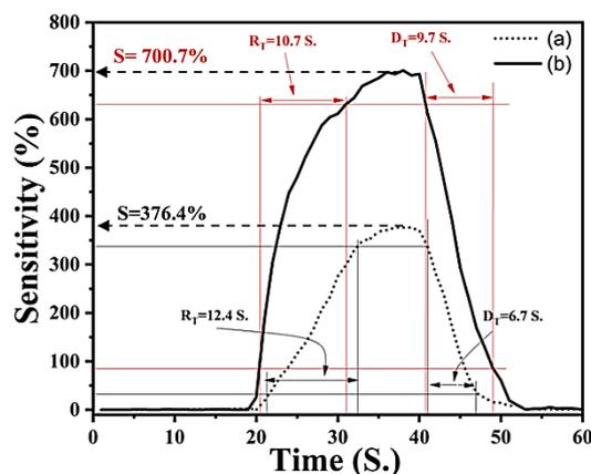
**Fig. 5: NH<sub>3</sub> sensing responses: (a) CuO nano-rods deposited on CuO thin layer, (b) CuO nano-rods with Ag nanoparticles**
