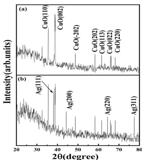
Fig. 3: XRD spectrum: (a) CuO nanorods deposited on CuO thin layer, (b) CuO nanorods with Ag nanoparticles.
