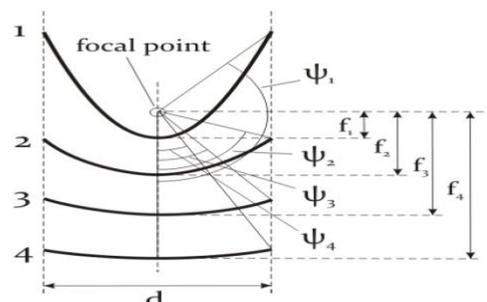
Figure (2) Relation between the focal length and the rim angle for a constant reflector diameter [16].
