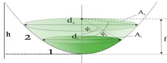
Figure (1) Geometrical dish parameters [16]
