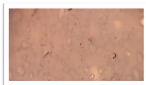
Fig. 11: Microscopic examination image of a section of a non-heat treated sample. (x400)
