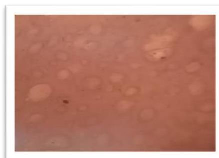
Fig. 3: Microscopic examination of a section of a thermally treatment sample for a period of (6hours) and with a treatment temperature ( T=70^{\circ}\text{C} ), It shows almost no defects. (x400).
