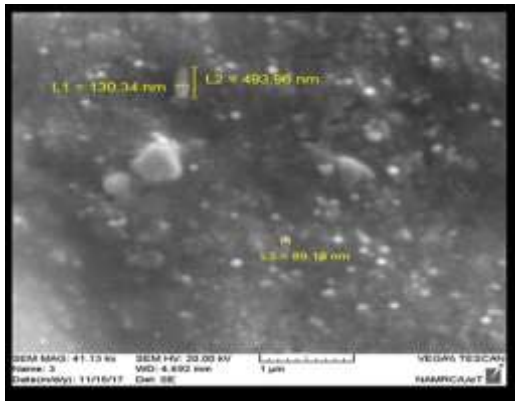
Figure (9) An image of the scanning electron microscopy (SEM) of part of the nanotubes (CNTs) in the Composite (F).
