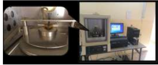
Figure (3) Thermal conductivity measuring device.
