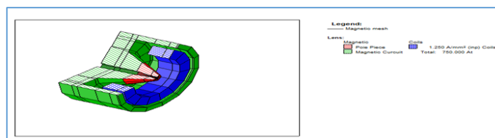
Fig. 2: 3-D of a magnetic unipolar prototype lens
