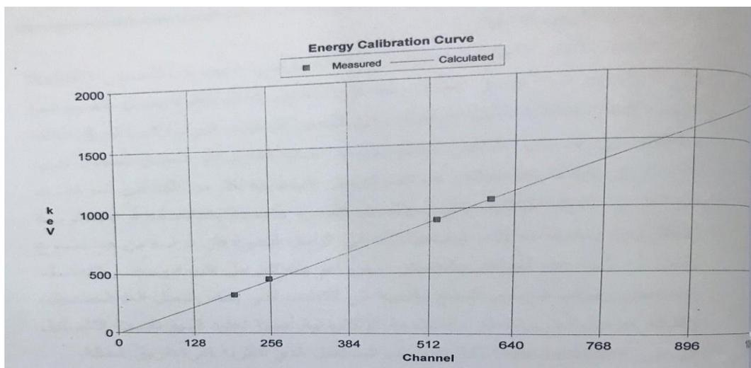
Fig. 3: Energy calibration curve of Compton peaks for the 2'x2' NE-213 detector.
