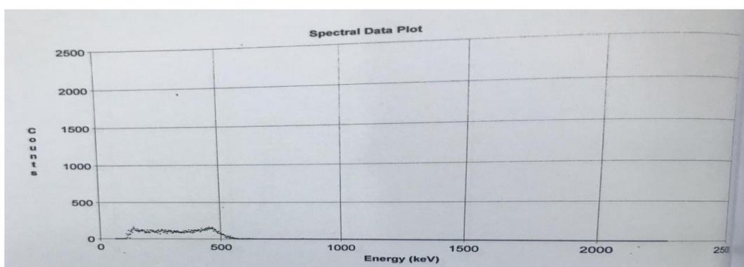
Fig.5: <sup>137</sup>Cs spectrum measured by the NE-213 detector.
