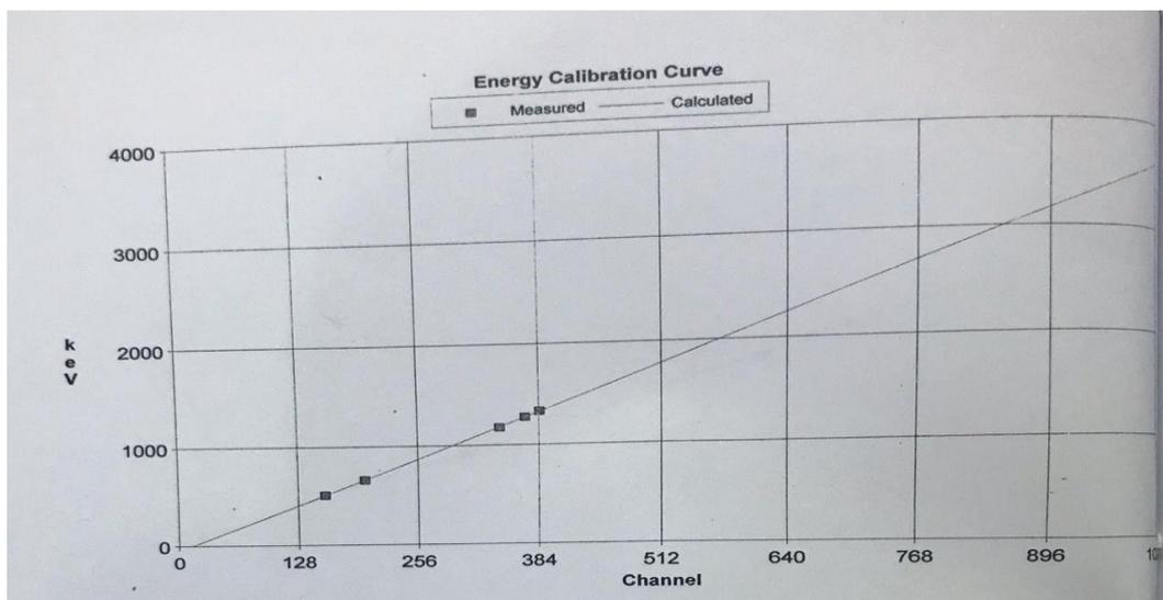
Fig. 1: Energy calibration curve of photo peaks for the 3'x 3' NaI(Tl) detector.
