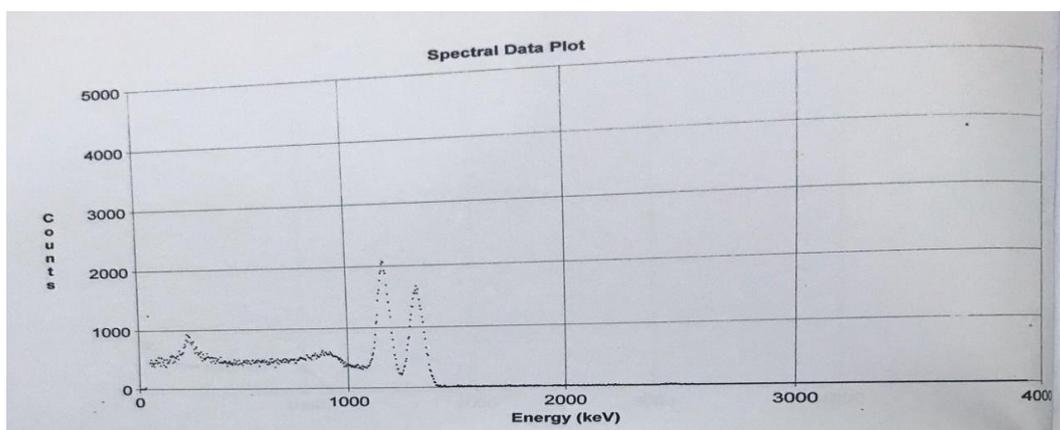
Fig. 7:  $^{60}\text{Co}$  spectrum measured by the NaI(Tl) detector.
