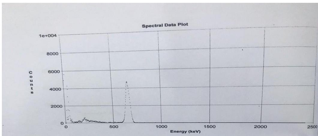
Fig. 6:  $^{137}\text{Cs}$  spectrum of the NaI(Tl) detector after subtracting Compton distribution.
