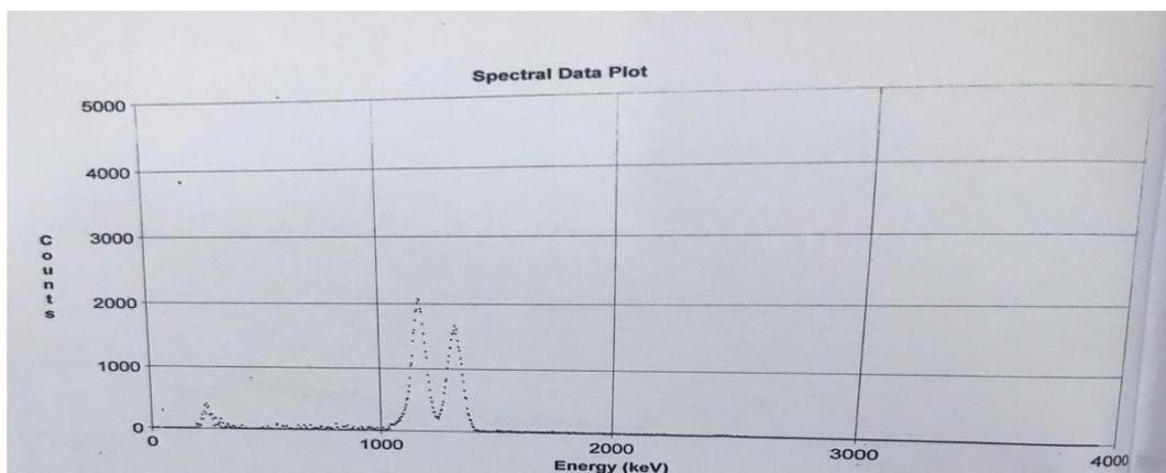
Fig. 9:  $^{60}\text{Co}$  spectrum of the NaI(Tl) detector after subtracting Compton distribution.
