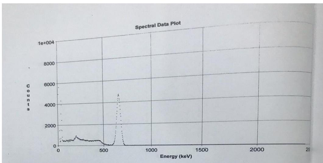
Fig.4: <sup>137</sup>Cs spectrum measured by the NaI(Tl) detector.
