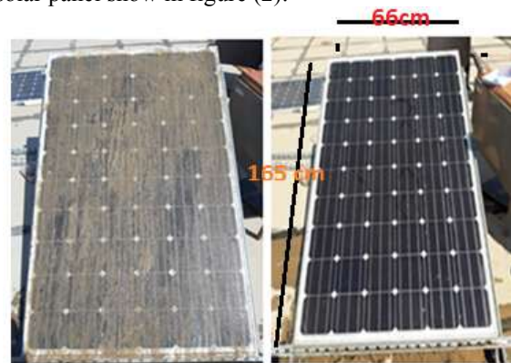
Fig. 2: left Solar panel with dust, right Solar panel clean.
