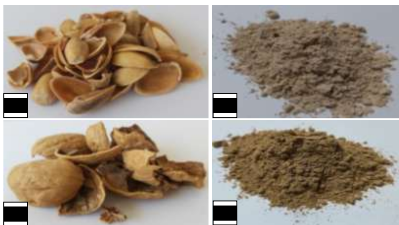
Fig. 1: a. pistachio shell b. pistachio shell powder c. walnut shell d. walnut shell powder
